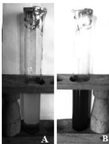
Figure 1: (A) Photograph of Plant extract and (B) AgNO 3 and Plant extract mediated silver nano particle solution after 2 hours of heating at 80 °C.
